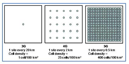
Figure 103. 5G Cell Tower Density Requirements
