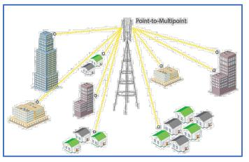
Figure 104. Point-To-Multipoint Fixed Wireless Networks
