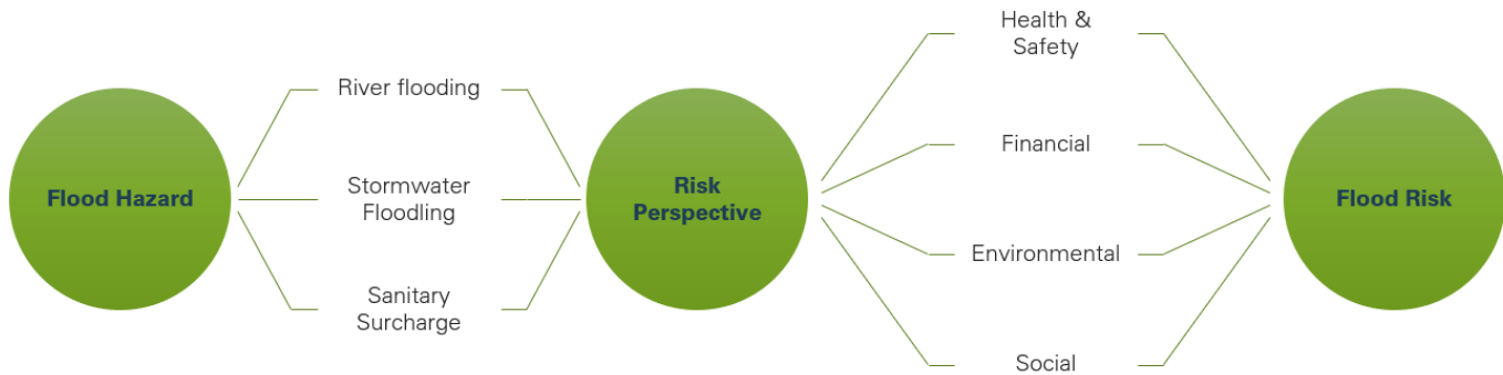
Figure 1: Flood risk is assessed with respect to three flood hazards: river flooding, stormwater flooding, and sanitary surcharge; for each flood hazard, risks are assessed with respect to the health & safety, financial, environmental, and social consequences.
